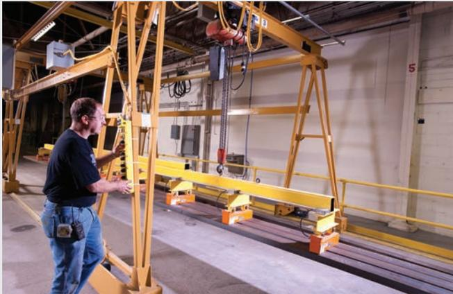
**A leading manufacturer** of commercial modular buildings changed its production process and needed a way to handle 6,500-pound bundles of steel. The steel's length and the plant's small size made the use of Combilifts™ unsafe and inefficient. The low ceilings required a custom-engineered, application-specific, material handling solution: two small Spanco Motorized PF-Series Gantry Cranes tied together with upper and lower steel channels and guided by double V-groove tracks.
