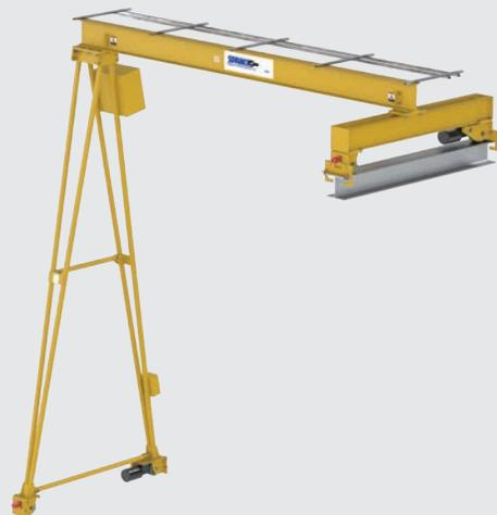
**Single Leg Gantries, Top-Running:** This configuration demonstrates a top-running end truck with one end of the crane traveling overhead, and one end supported by a single leg and trackless power drive.
