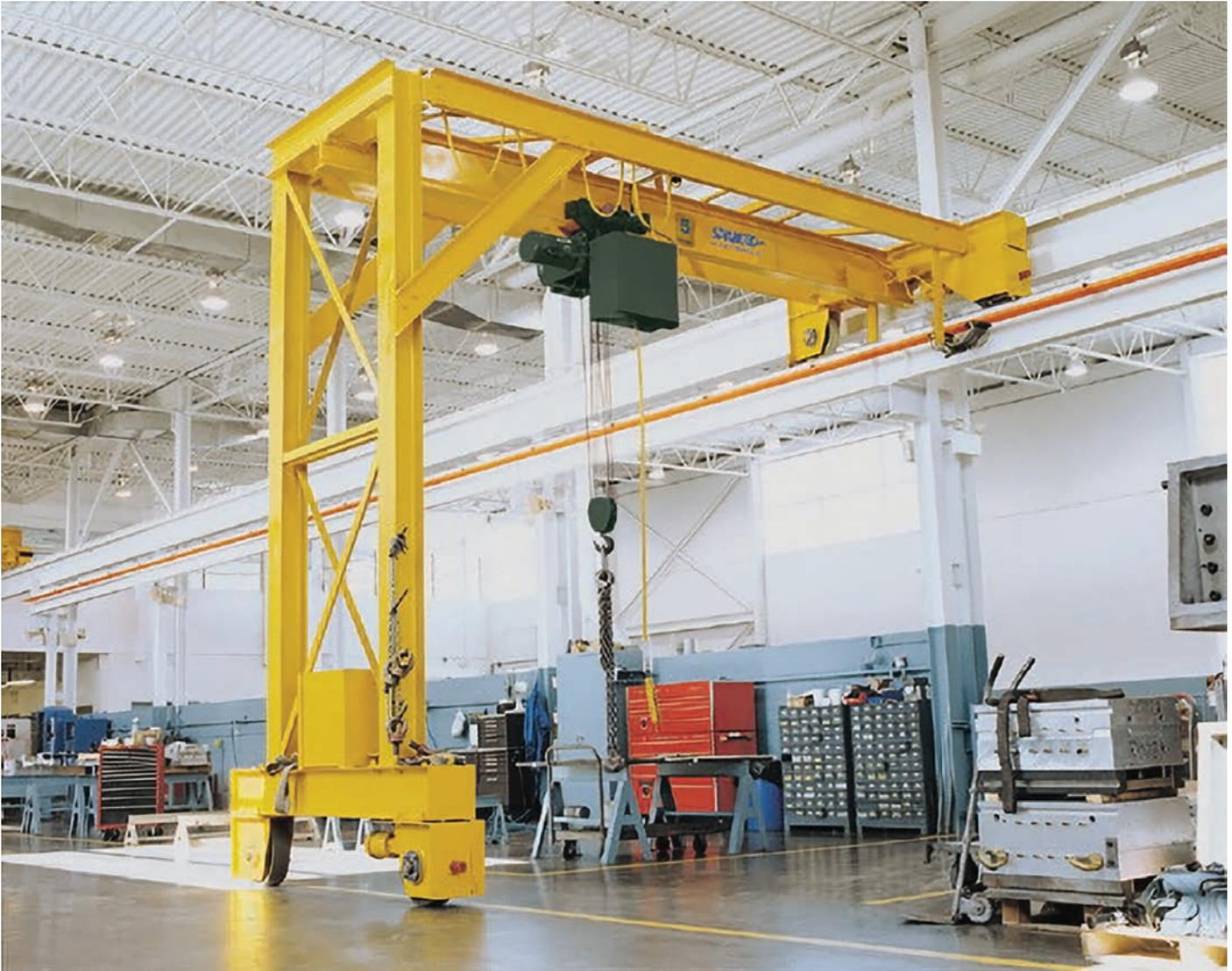
Motorized 5-ton Wide-Flange Single-Leg Gantry Crane
