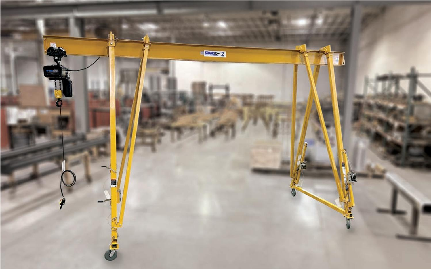
T-Series Gantry Crane in a cantilever configuration
