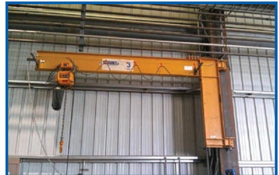
*Spanco Wall-Mounted Jib Cranes easily fold out of the way of larger overhead cranes for a flexible workflow.*
