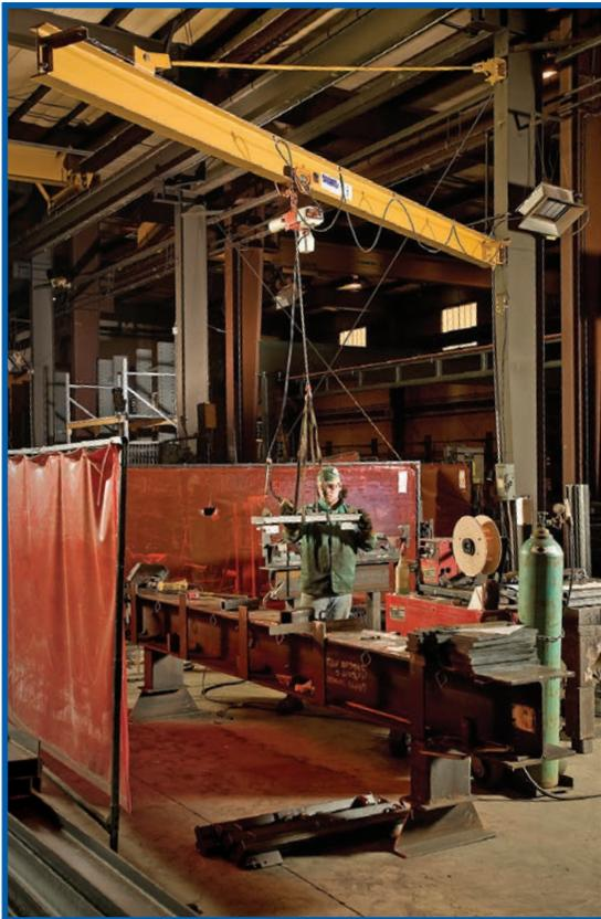
*A Spanco 301-Series Wall-Bracket Jib Crane*
