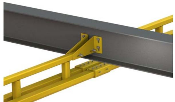
**Save Headroom:** A unique option to save headroom is to mount the header beam through the truss of the runway track, if the inside of the truss is tall enough to fit the header. For example, for four-column systems, you can mount the top tube of the runway track to the top of the header and sit the truss between the columns.
