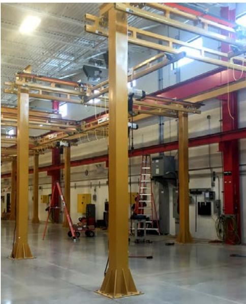
**Inverted-L Columns:** Inverted-L columns can be used for applications that require angled headers or uneven columns. These columns don't require a cross header, so the columns on opposite sides don't need to line up.
