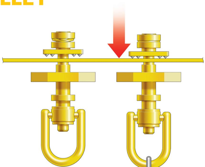
Hardened steel teeth activate and arrest any trolley movement when any force greater than 80 pounds, including the weight of the self-retracting lanyard, is applied.
