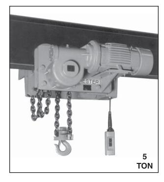
We offer a complete line of worm gear driven, electric, low headroom trolley hoists. These hoists are equipped with case hardened load chain and are available in models to lift and move loads from 1 to 24 tons. Choices of plain push/pull, hand-geared or motorized trolley drives are available to meet a variety of applications.
