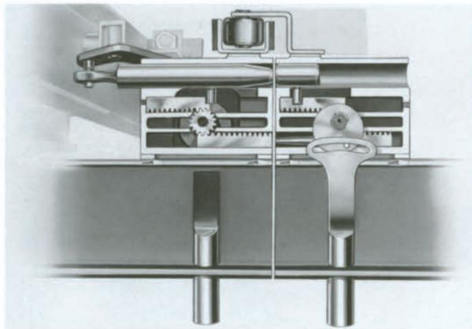
**HAND-OPERATED LATCH** is used for light and medium duty crane and monorail operations, these latching mechanisms give positive track alignment needed for smooth operation of trolley wheels through the latching point.
