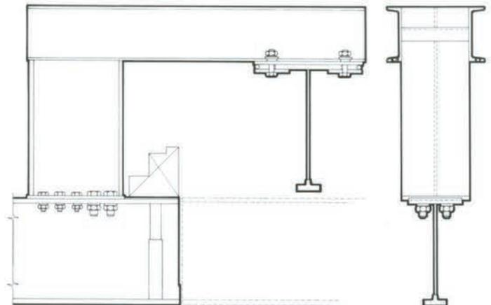
**SPUR TRACK** support is used to provide smooth passage of trolley wheels over the transfer joint from crane to monorail. Since the end of the spur track is supported on the crane runway, any deflections at the ends of the crane bridge and spur track are equalized. No other support of the spur track should be provided close to a spur track support since this would upset its equalizing effect.
