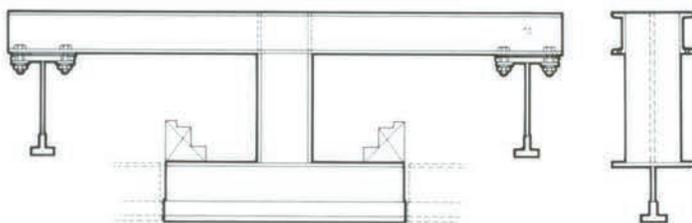
**TRANSFER SECTION** mounts on adjacent crane runways providing a means for a load to move from one crane to another across a building column line without costly rehandling. Any deflections are equalized, permitting smooth passage of the trolley wheels.
