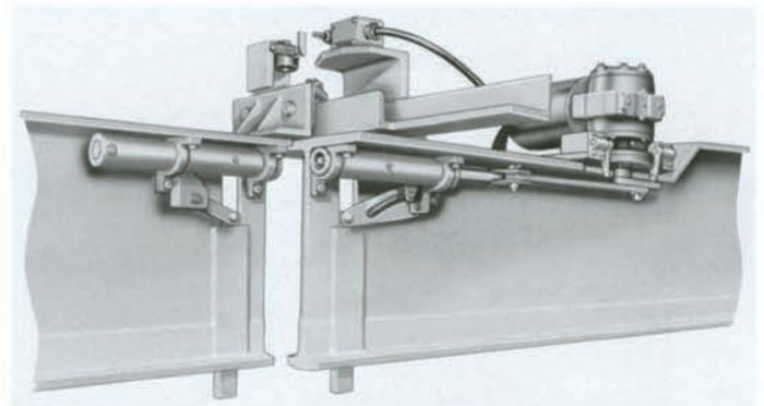
**MOTOR-OPERATED LATCH** is used for heavier duty crane and monorail operations. This latch is equipped with a channel-shaped guide which functions with a heavy roller mounted on the block to allow latching and proper track alignment.
