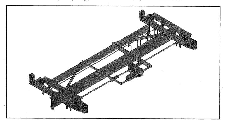
The Louden Series 503 center drive crane is offered in capacities of 1 through 5 tons, with spans to 58 feet. Standard bridge speeds are 75 and 135 F.P.M., single speed. Optional travel speeds (single speed) are 50, 110, 165, 190, and 225 F.P.M. Other optional speeds are 2-speed, and variable speed. High speeds listed above.
