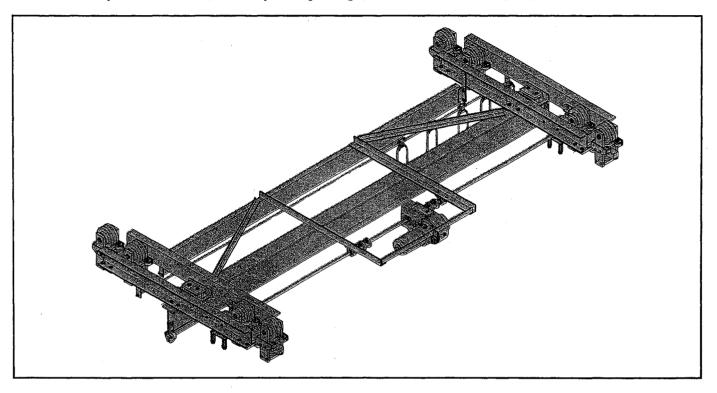
The Louden Series 503T center drive crane is offered in capacities of 5 through 10 tons, with spans to 60 feet. Standard bridge speeds are 75 and 135 F.P.M., single speed. Optional travel speeds (single speed) are 50, 110, 165, 190 ,and 255 F.P.M. Other optional speeds are 2-speed and variable speed. High speeds listed above.
